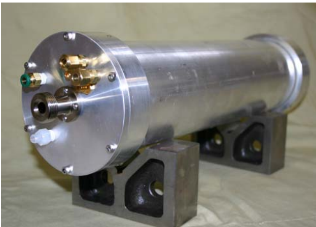
Figure 1. Tubular containment pressure vessel.
